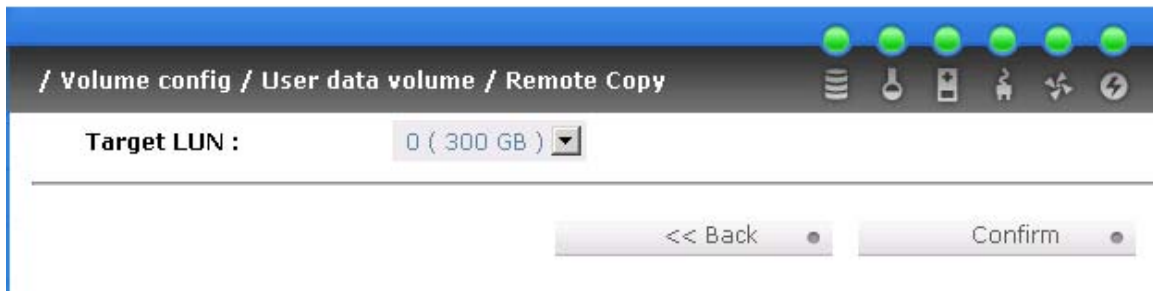
Figure 4.5.3 (Figure 4.5.3: select the target UDV LUN, the target UDV capacity must be equal or larger than the source UDV capacity.)
